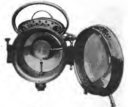
FIG. 4.—BESNARD LAMP WITH ECLIPSING DISC LOWERED INTO POSITION.
